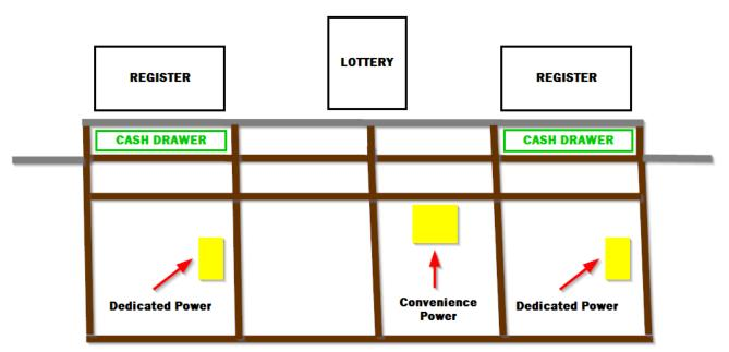
Add a mark either at the floor or from above for marking the location of the data cable entrance. Some designs only have 3 cabinets not the 4 shown here.
